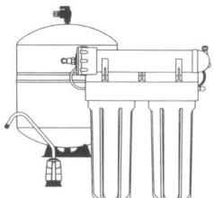
IMPORTANT! We do not recommend that these reverse osmosis systems be used with water in excess of 10 gpg (171 mg/L) hardness. Doing so will cause lime scale to build up on and plug the membrane.
