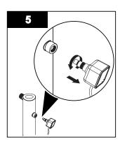
Remove the UV sensor by grasping the body of the sensor and rotating it counter-clockwise.
