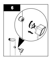
Install the new UV sensor until a water-tight seal is achieved.
