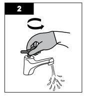
Open a tap downstream of the UV unit to release pressure. Then, close this tap.
