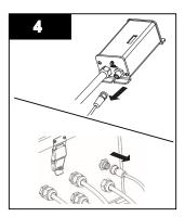
Disconnect the UV sensor from the controller by disconnecting the sensor cable.
